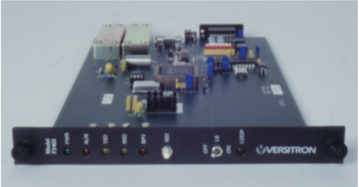
FIGURE 1. OVERALL VIEW, F2400 FIBER OPTIC MODEMS
